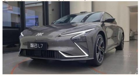
Coming to the side, the car looks light and dynamic with its gently sculpted sides. For reference, the IM L7 has a dimension of 5098/1485/1960mm with a 3100mm wheelbase and a drag coefficient of 0.21cd.
