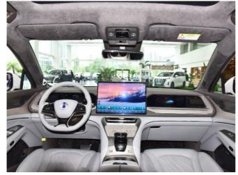
Inside, the interior has a 15.6-inch touch screen, a double-spoke flat-bottom multifunctional steering wheel, and a floating full LCD instrument panel.
