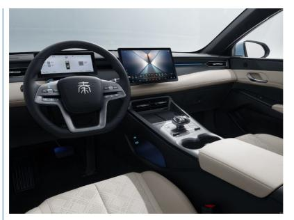
**Top Overview** Consumption: 13.6 kWh/100km Battery type: LFP Battery capacity: 15.8 kWh Drive: Front Top speed: 180 km/h Acceleration 0-100 km/h: 7.6 sec Peak torque: 210 Nm Number of seats: 5 L/W/H: 4780/1837/1515 mm Wheelbase: 2718 mm Assisted Driving Chips: NVIDIA DRIVE Orin N Vehicle system memory: 8 GB ADAS: DiPilot Body type: <u>Sedan</u> Fuel type: PHEV
